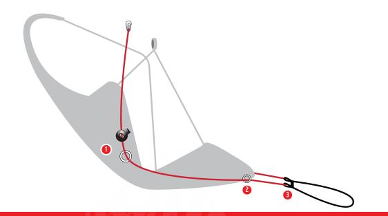
CAUTION: Make sure that the speed system is not too short. The front risers of your paraglider must not be pulled down in normal (unaccelerated) flight.
